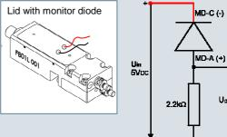
Monitor diode connection (bias mode): Red wire = cathode photo diode (-) Black wire = anode photo diode (+) Resistor is not included. The wires come out of the lid.
