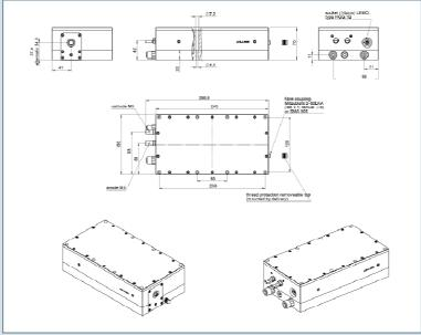
Module with macro channel water cooling
