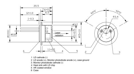
All devices are pretested and will be delivered with the certificate including measured laser characteristics. For safety, unpacking, handling, mounting, operating and warranty issues, please read attentively our "Operating manual".
